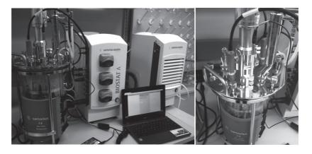
**Figure:** Sartorius Biostat A MO UniVessel 5-L Fermenters. These fermenters are dedicated for Upstream Biotechnology Processes course.
